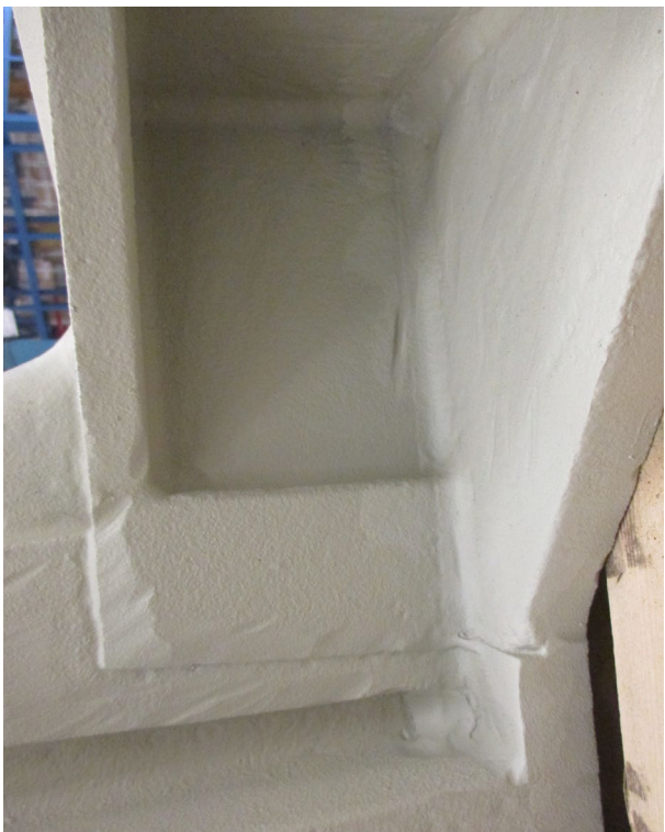
constriction at the transition, machining marks
